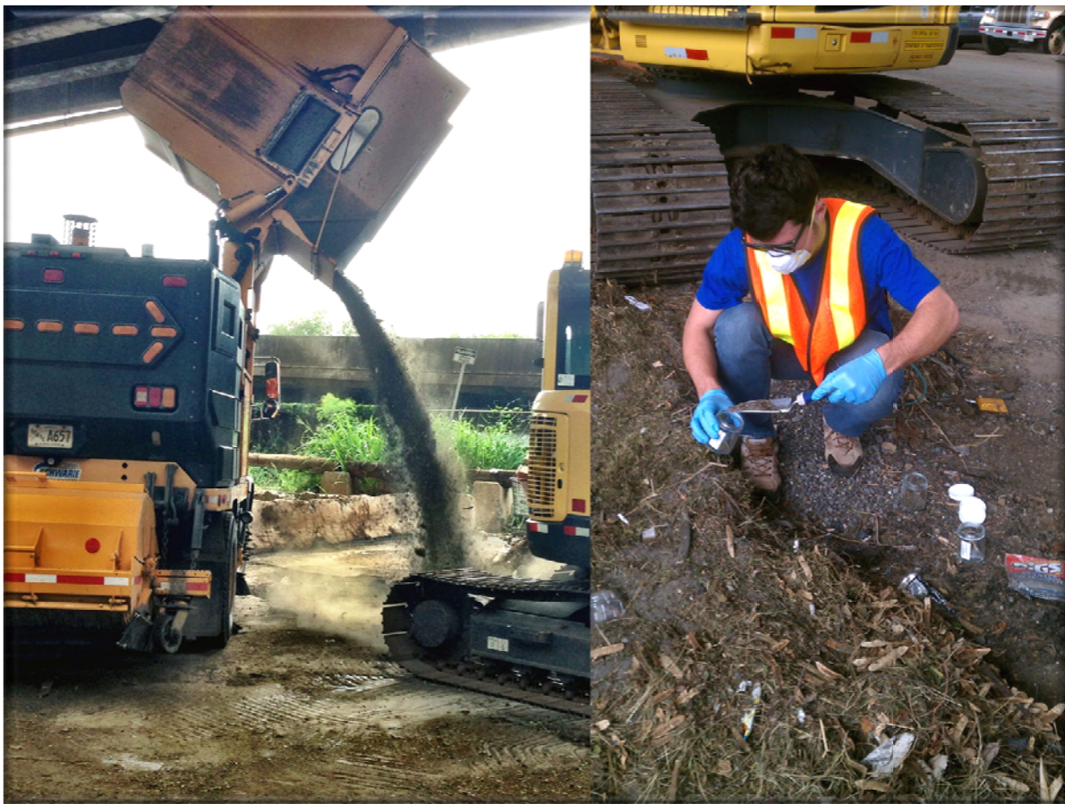
Street sweeper dumps debris at Keahi Baseyard Transfer Station (left), and Inspector obtains samples of the street sweeping debris for the Debris Cleaning Assessment (right).
