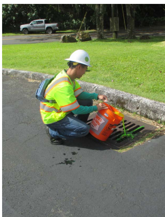
An inspector performs a dye test to verify the connectivity of the private drainage structure to the DOT-HWYS MS4.
