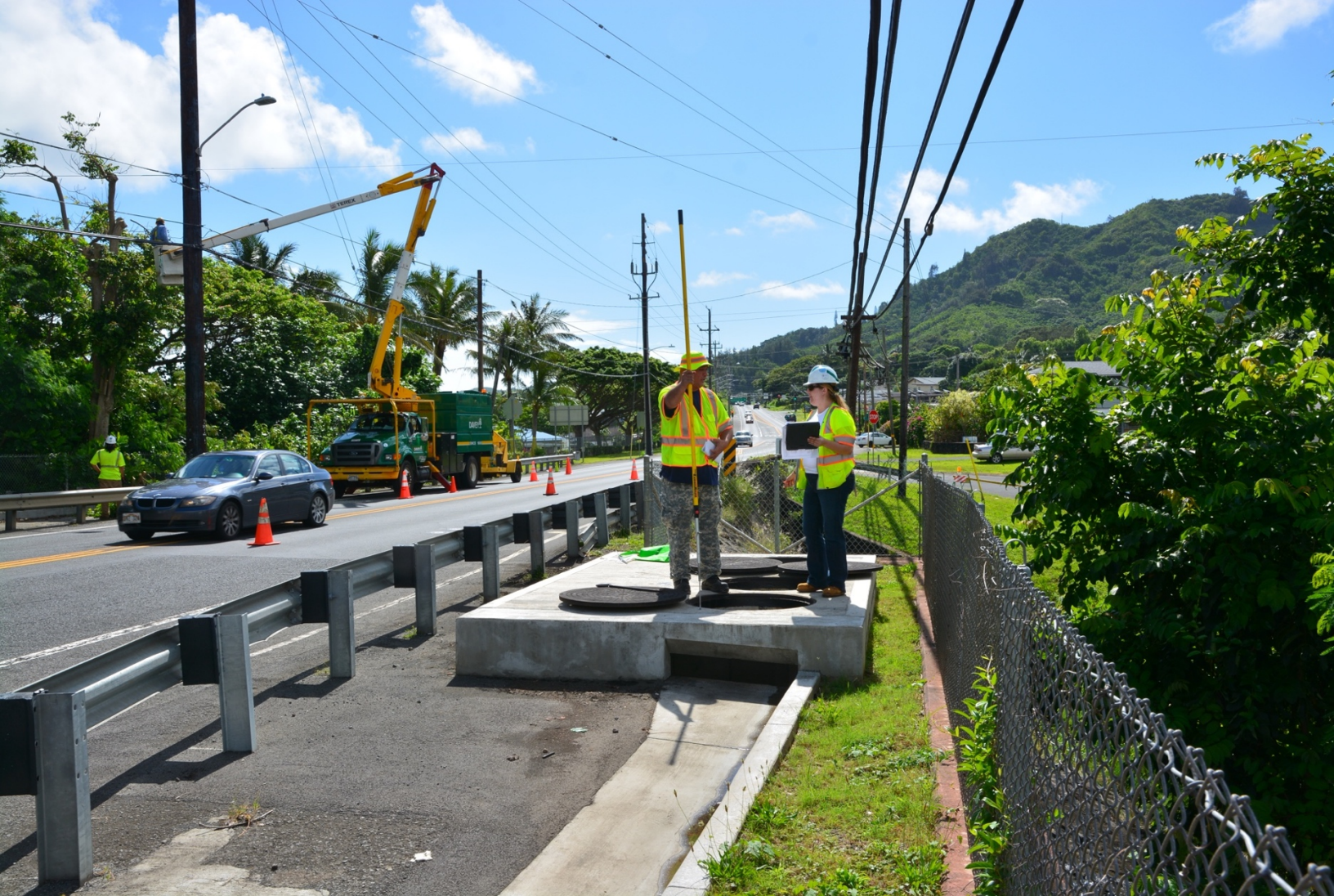
Inspectors collect grab samples from a water polisher along Kaneohe Bay Drive, Kaneohe, Hawaii.
