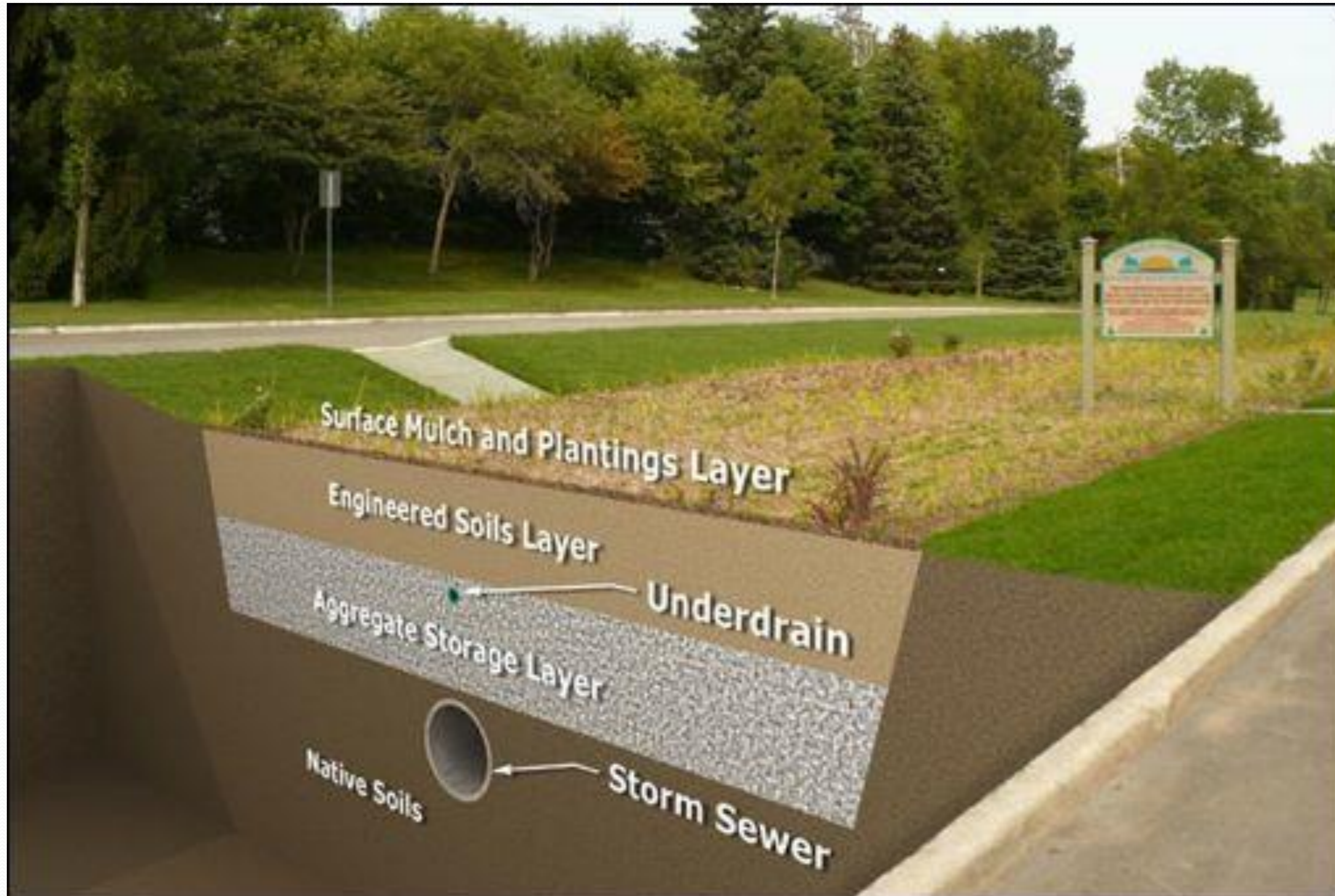
Bioswale or “Enhanced Swale”
