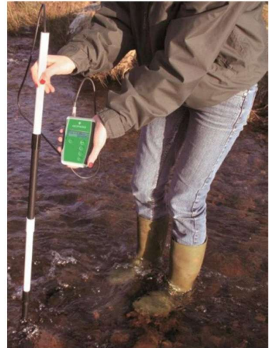
Example water flow meter and its use in the field. (Photos courtesy of Hydrometag)
